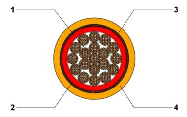
1 Core 120 mm<sup>2</sup> Conductor: stranded bare copper 589 x 0.51 mm D Insulation: RADOX 155 D: 18.00 ± 0.30 mm
